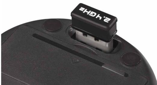
USB nano receiver conveniently stowed on the back.
